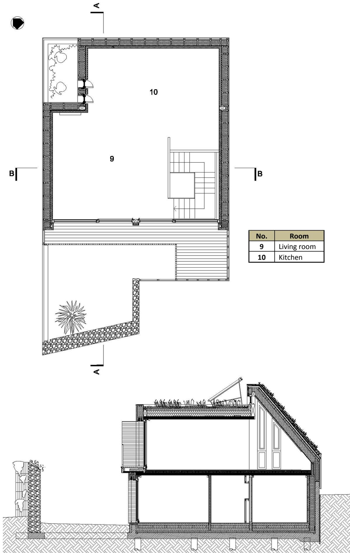
Figure 12- First floor and cross-section A-A, S=1:100 (Bere: architects, 2009)
