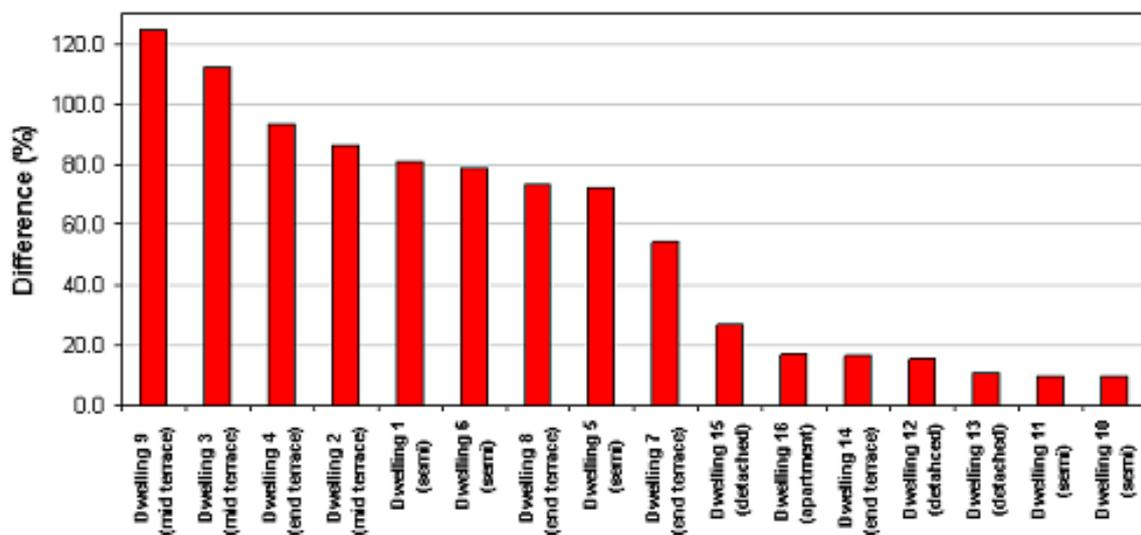
Figure 6- Difference (%) between measured and predicted whole house heat loss in 16 new low energy dwelling (Wingfield, et al., 2009, cited in GHA, in press, p. 24)
