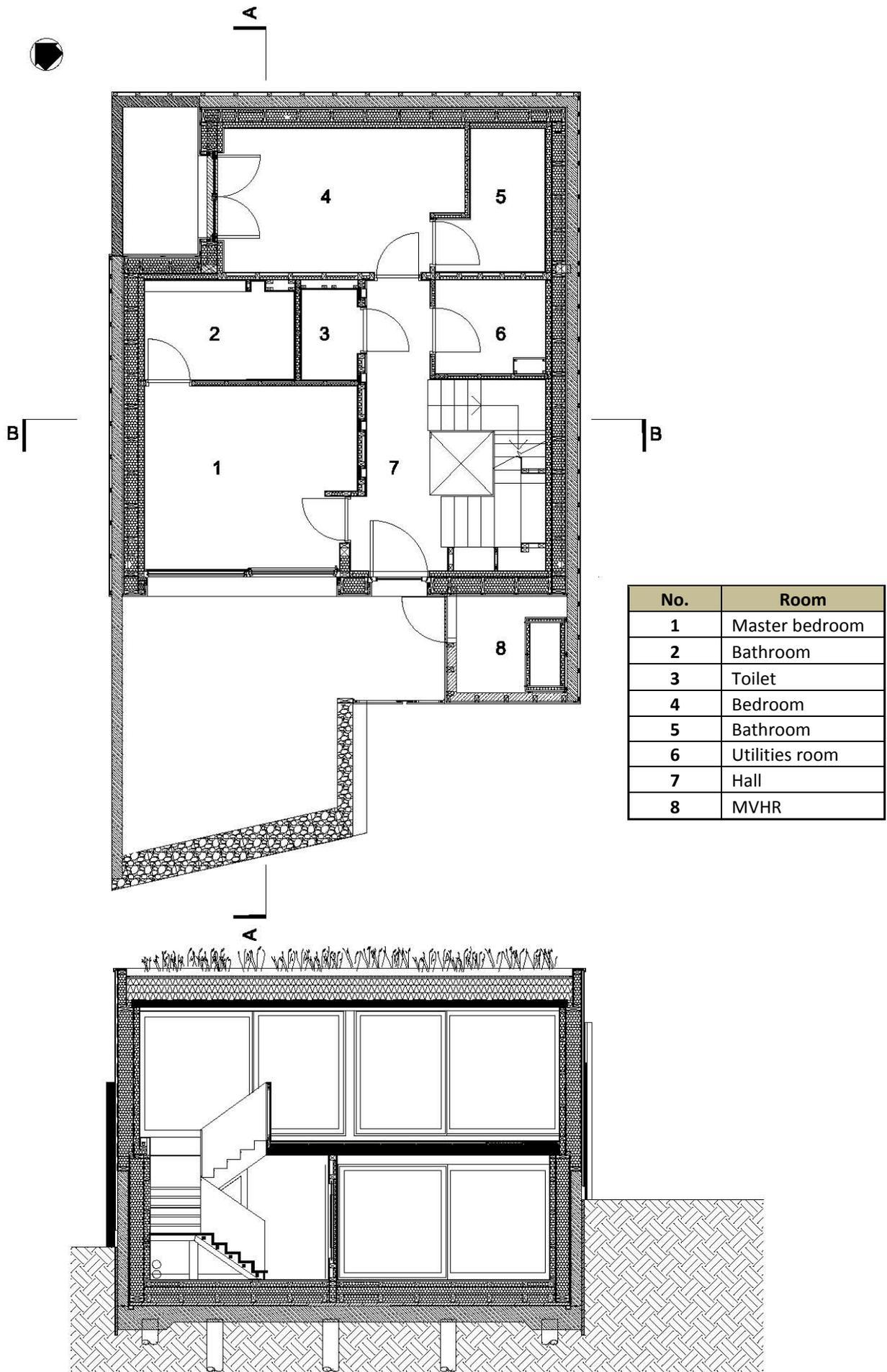
Figure 11- Ground floor and cross-section B-B, S=1:100 (Bere: architects, 2009)
