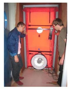
Figure C-13. Building-time blower-door test, the value n50 = 0.47 1/h was reached.
