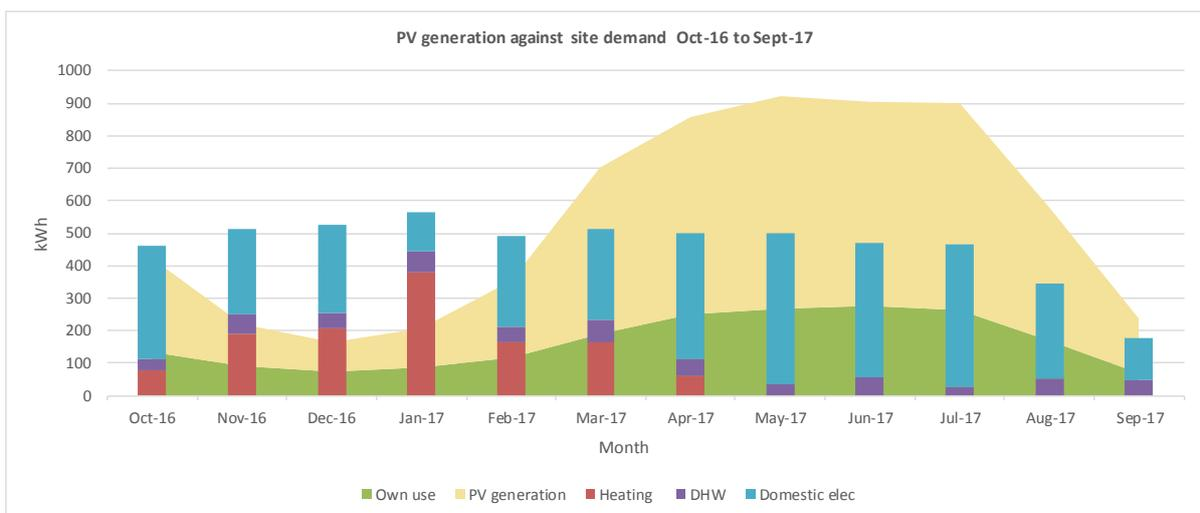
**Figure 12. Showing PV electricity generation (ramped down pending battery storage, to avoid overloading the grid) and total electricity demand of Lark Rise between Oct-16 to Sep-17**
