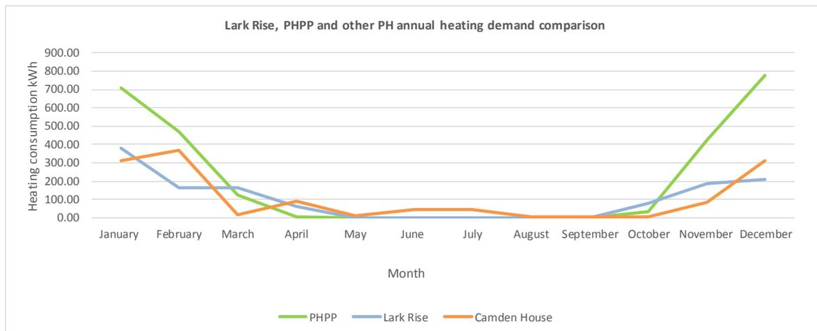
**Figure 7. Lark Rise average heating consumption (between Oct-16 and Sept-17) compared to PHPP and Camden House (between Oct-12 and Sept-13)**
