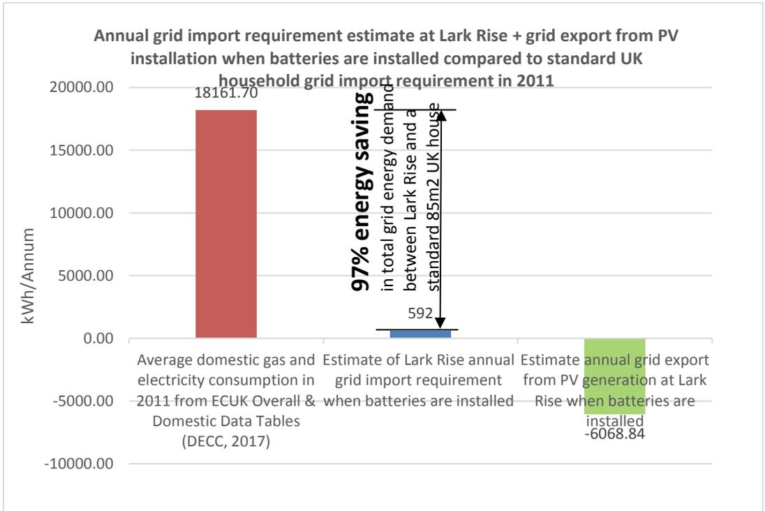
Figure 14. Grid energy requirements – UK average domestic gas and electricity consumption in 2011 from ECUK Overall & Domestic Data Tables (DECC, 2017) and Lark Rise compared. Figure 15 (below) as above but shown per square metre.
