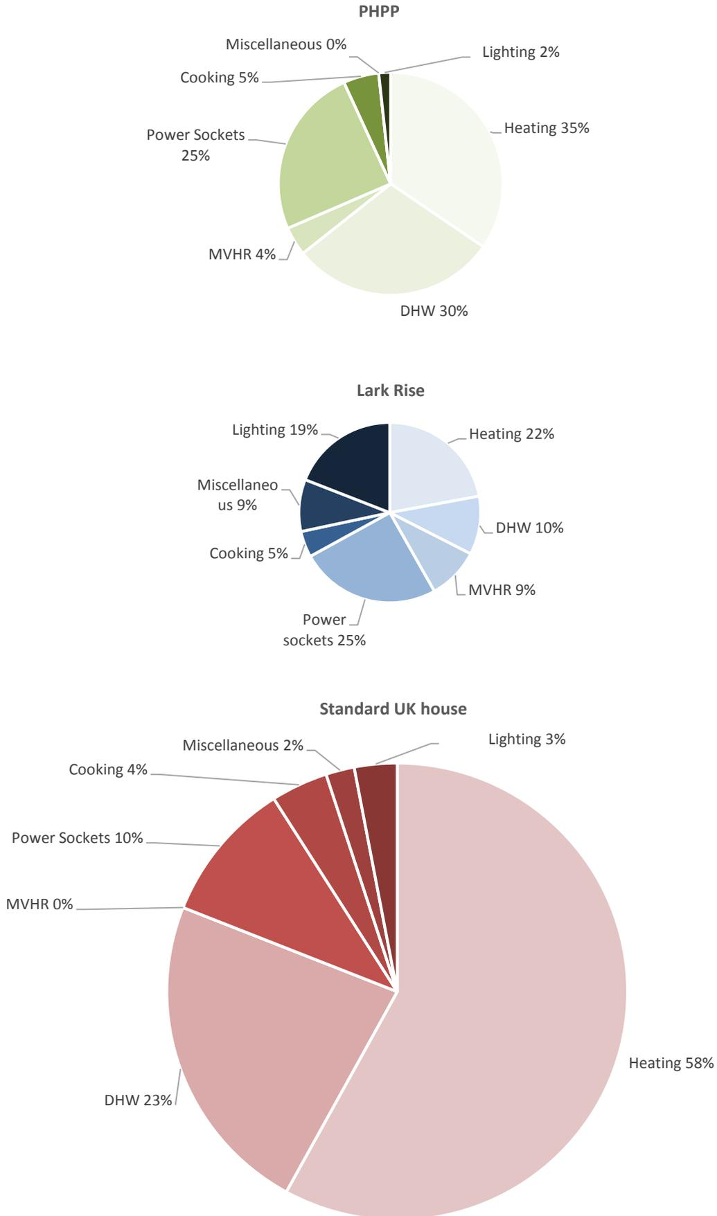
**Figure 4. PHPP design estimate, UK standard house and Lark Rise average total final energy consumption, (between Oct-16 and Sept-17). Percentages of by end use of a UK standard home have been taken from Figure 3-1 UK of Domestic energy use by fuel type and by end use shown in page 47 of the thesis 'A specification for Measuring Domestic Energy Demand Profiles' (Svehla, 2011) which is based on ECUK tables of 2010 of BEIS.**
