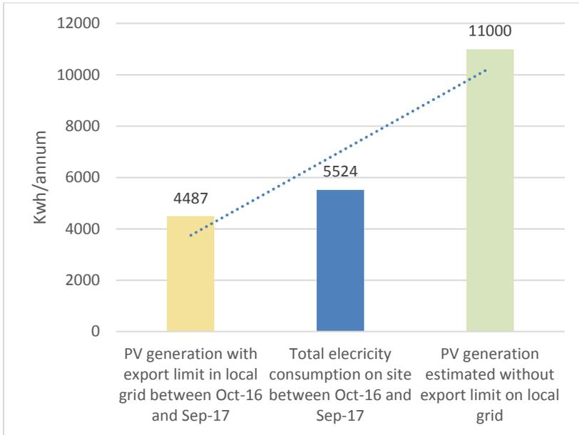
**Figure 11. Actual total annual PV generation a Lark Rise between Oct-16 and sep-17 (in temporary throttled-down mode to limit export below 3.8kW) against actual demand on the same period and PV generation estimate by Energelio (once full PV generation capacity can be enabled) in their Self-consumption report of 29<sup>th</sup> of April 2016**
